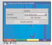
Now use the arrow keys up/down to select the type of scan you wish to perform, and confirm by pressing OK.
